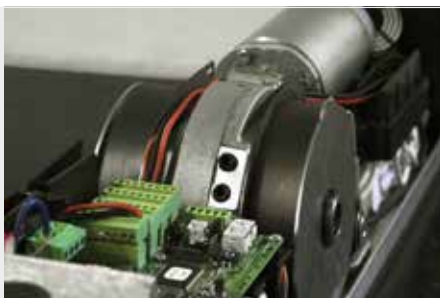
Full Power or Low Energy modes can be easily selected from the electronic board.
